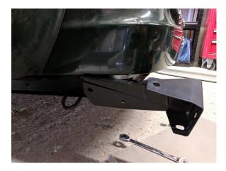
However, this proved to not work – the washers raising the body (to accommodate the alternator) got in the way and it was not possible to secure the bumper effectively.
