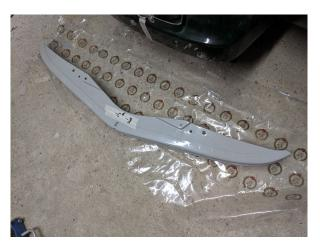
3:00am solution. Invert the bumper so that the wider bit sits under the body, the narrow bit wrapping around above. Putting it into practice proved impossible as the bumper would not sit back far enough to be bolted to the chassis.
